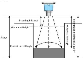
As picture above, the instrument probe send wave hit level then reflected back to probe, after received wave, the probe calculated the time from sending wave to receive, get measuring distance L, the height of instrument installation TH minus the measuring distance L, then will get the current level height H.
